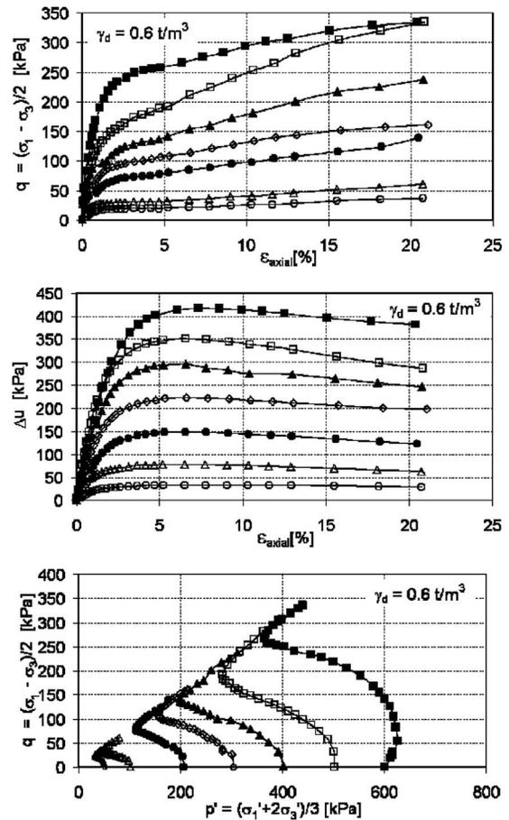
**Fig. 14.** Stress-strain curves, pore pressure, and effective stress paths obtained in CIU triaxial test on reconstituted specimens of diatomaceous soil ( $1 \text{ t/m}^3 = 9.8 \text{ kN/m}^3$ )
