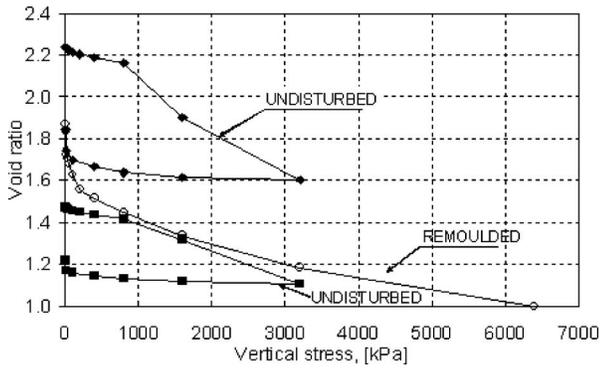
**Fig. 12.** Consolidation results of diatoms on undisturbed and reconstituted specimens
