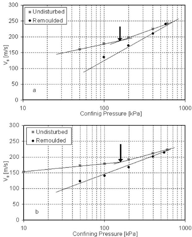
**Fig. 9.** Shear wave velocities measured on undisturbed and remoulded samples on (a) Santa Barbara; (b) Chillán volcanic ash soils
