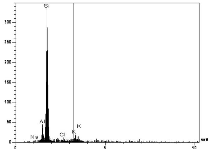
Fig. 11. EDX spectrum analysis of diatomaceous soil of this study
