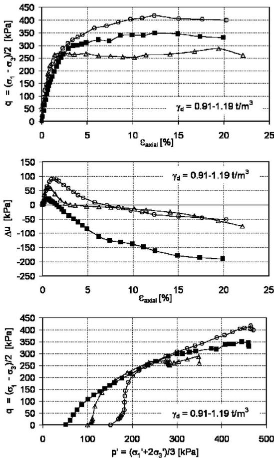
**Fig. 13.** Stress-strain curves, pore pressure, and effective stress paths obtained on CIU triaxial tests on undisturbed specimens of diatomite ( $1 \text{ t/m}^3 = 9.8 \text{ kN/m}^3$ )
