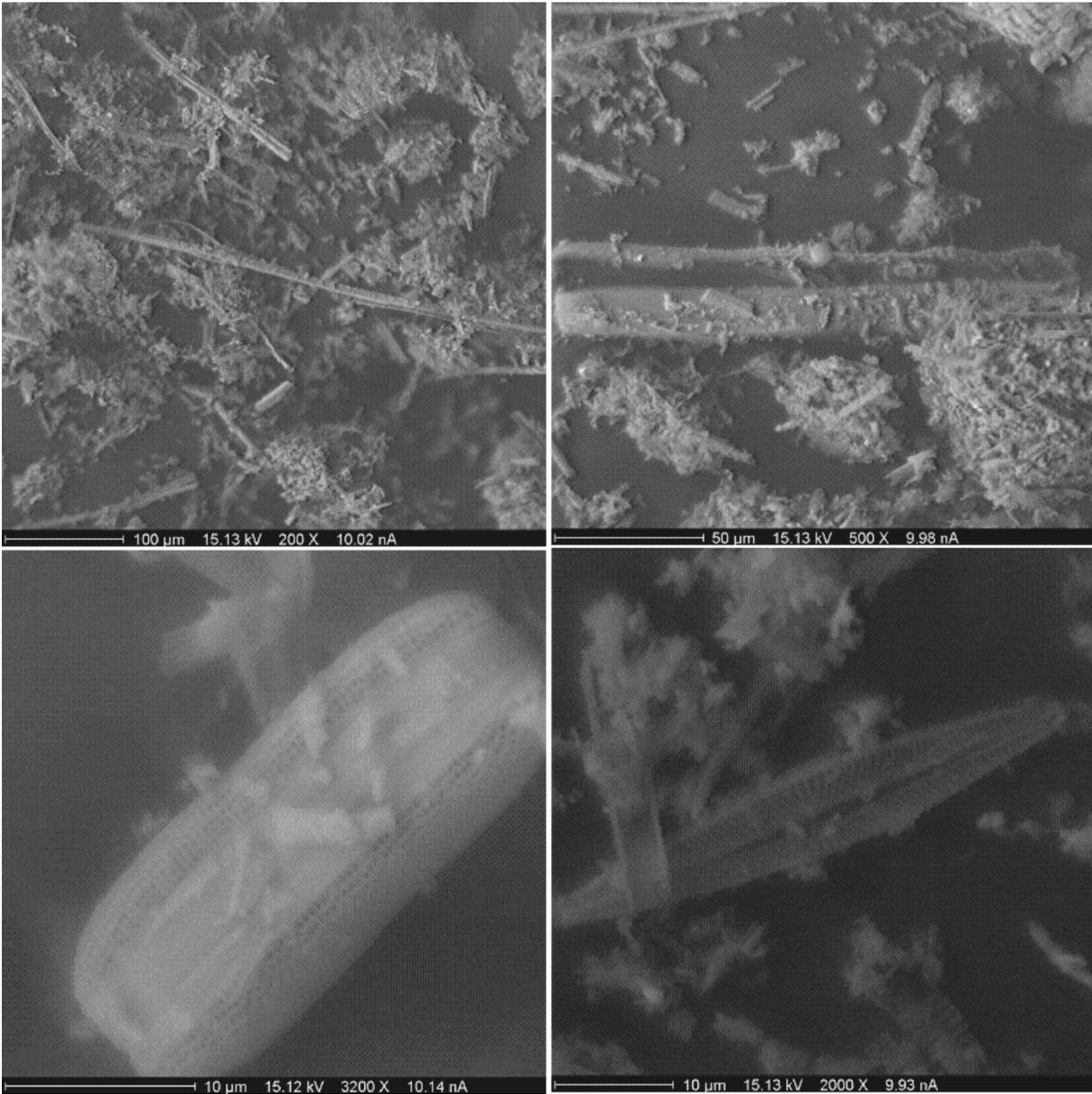
Fig. 10. Particle shape of diatomaceous soil of this study
