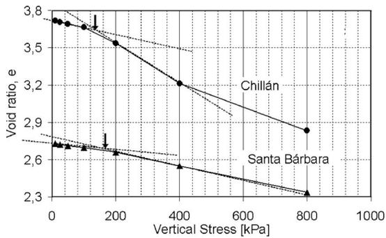
Fig. 5. Consolidation test results on undisturbed samples
