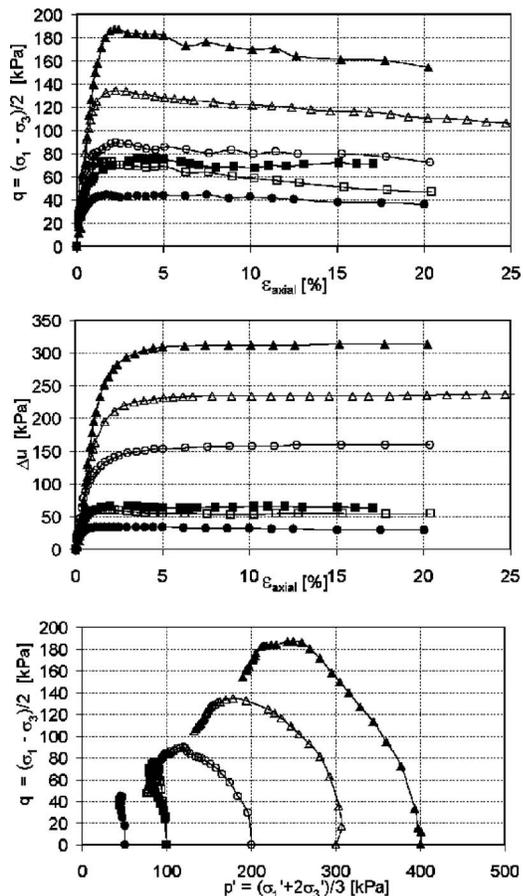
Fig. 6. Triaxial test results on undisturbed specimens of Santa Barbara volcanic ash soil
