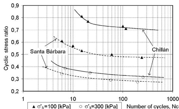
Fig. 8. Effect of confining pressure on cyclic strength of undisturbed specimens of Chillán and Santa Barbara volcanic ash soils
