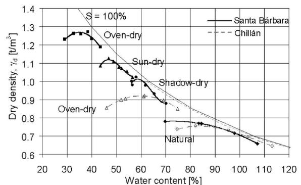
Fig. 4. Effect of drying on the Proctor compaction test
