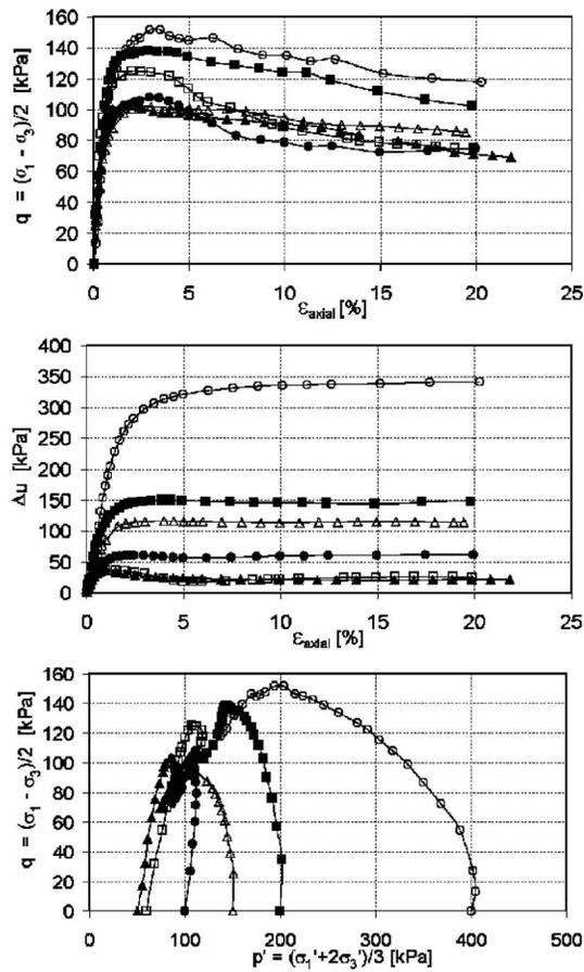
Fig. 7. Triaxial test results on undisturbed specimens of Chillán volcanic ash soil
