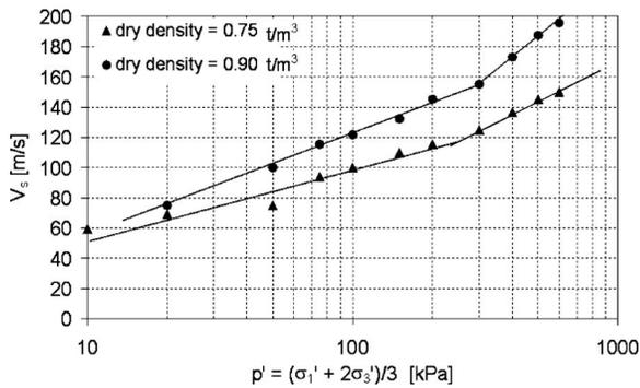
**Fig. 15.** Effect of density on shear wave velocity on reconstituted specimens of diatomaceous soil ( $1 \text{ t/m}^3 = 9.8 \text{ kN/m}^3$ )
