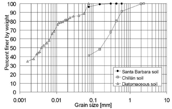
Fig. 2. Grain size distribution curves of tested soils
