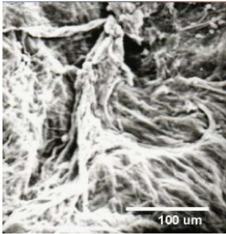
**Fig. 1.** Electron-microscope photograph of imogolite particles
